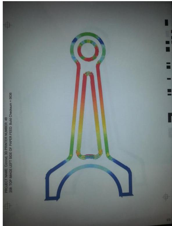
*Paper layer from Mcor Technologies' 3D printer*
